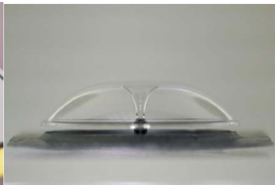
Figure 4. Micro-glassblown wineglass structure with 4.2 mm diameter, 50 \mu\text{m} thickness and 300 \mu\text{m} central stem.
